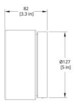
RP-WS Ripple Sconce Dimension (Rotate 90 degrees for flush mount version)
