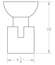
Made of cold rolled steel, the table is finished in a light antique brass with a dark antique brass block base. The contrasting finishes accentuate the interlocking shapes.
